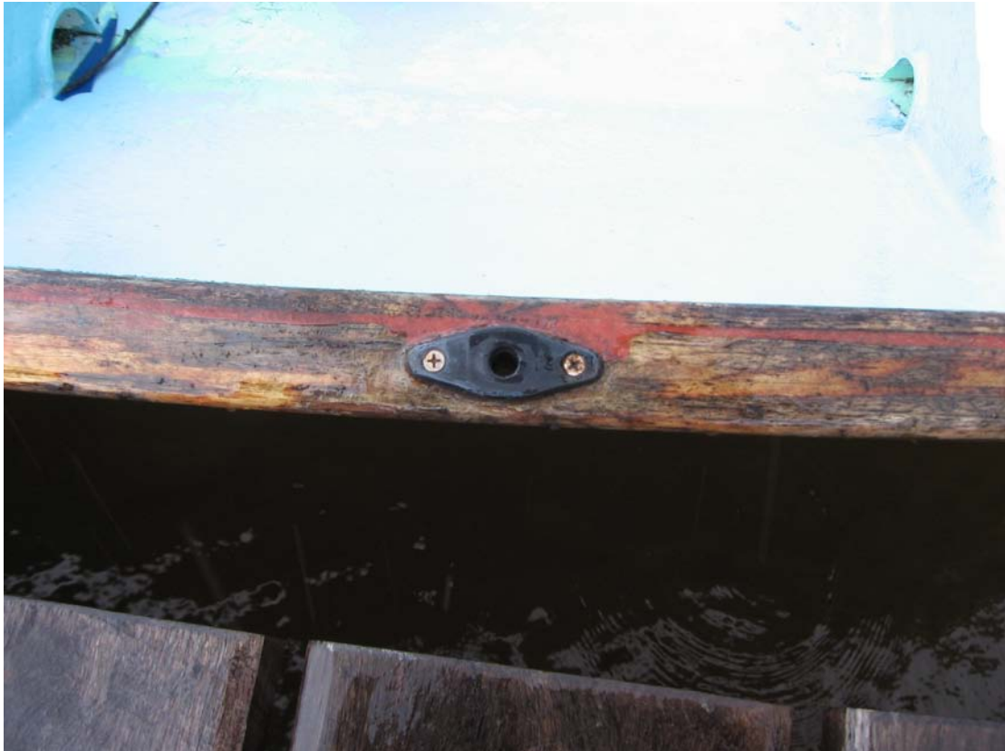
Socket worn down but not out after 5 years of use (The down wear can be obviated with a stainless washer)
