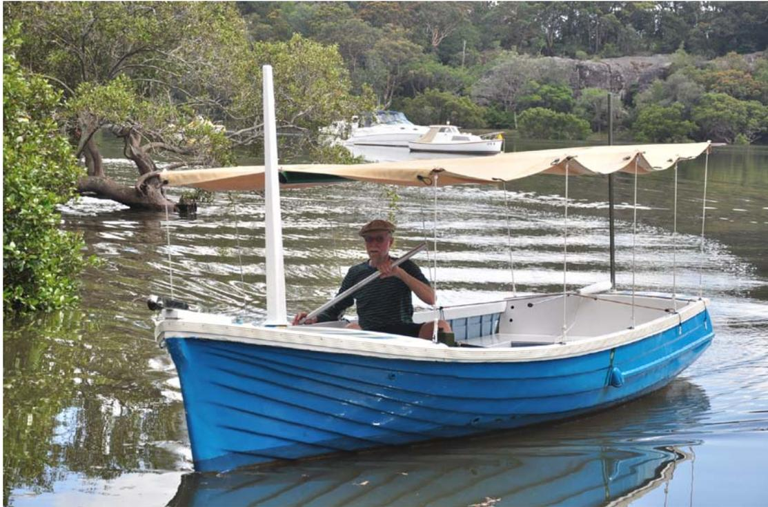
**My beautiful “Brunkenkunjekrub” could not exist today without the sistered ribs, replaced planks and a layer of fiberglass to support its tired timbers. Is it “traditional”?**
