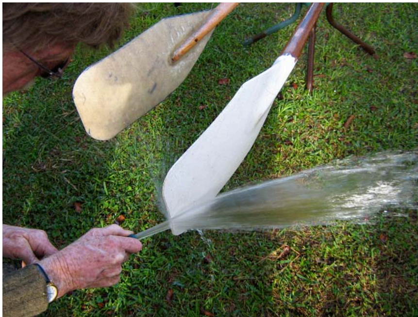
The water does not attach to the rear of a more conventional blade.
