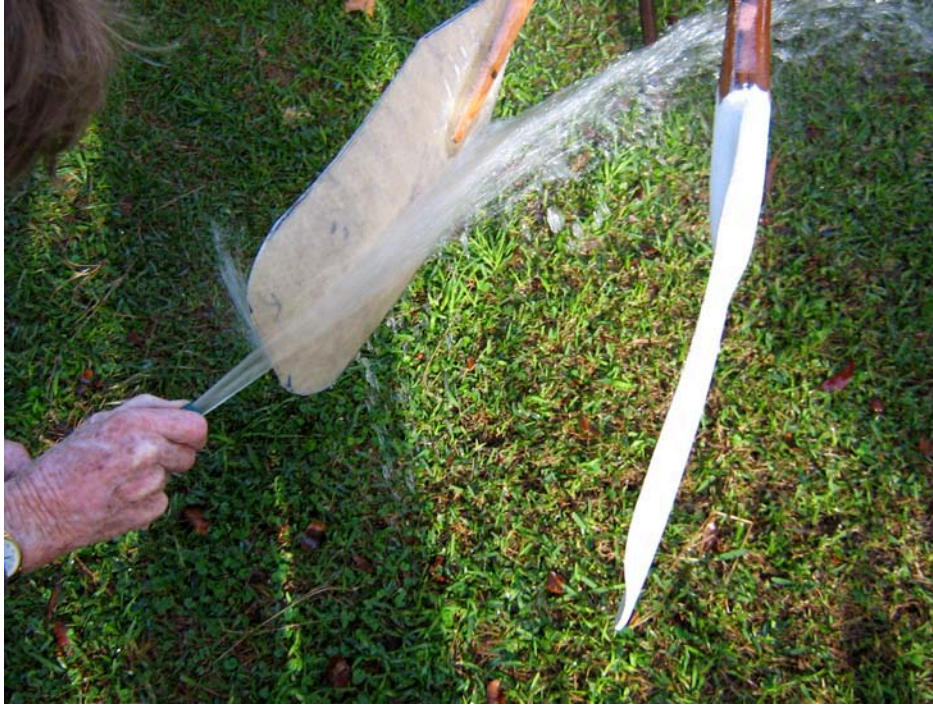
The water attaches to the rear of the prototype for at least part of its length.
