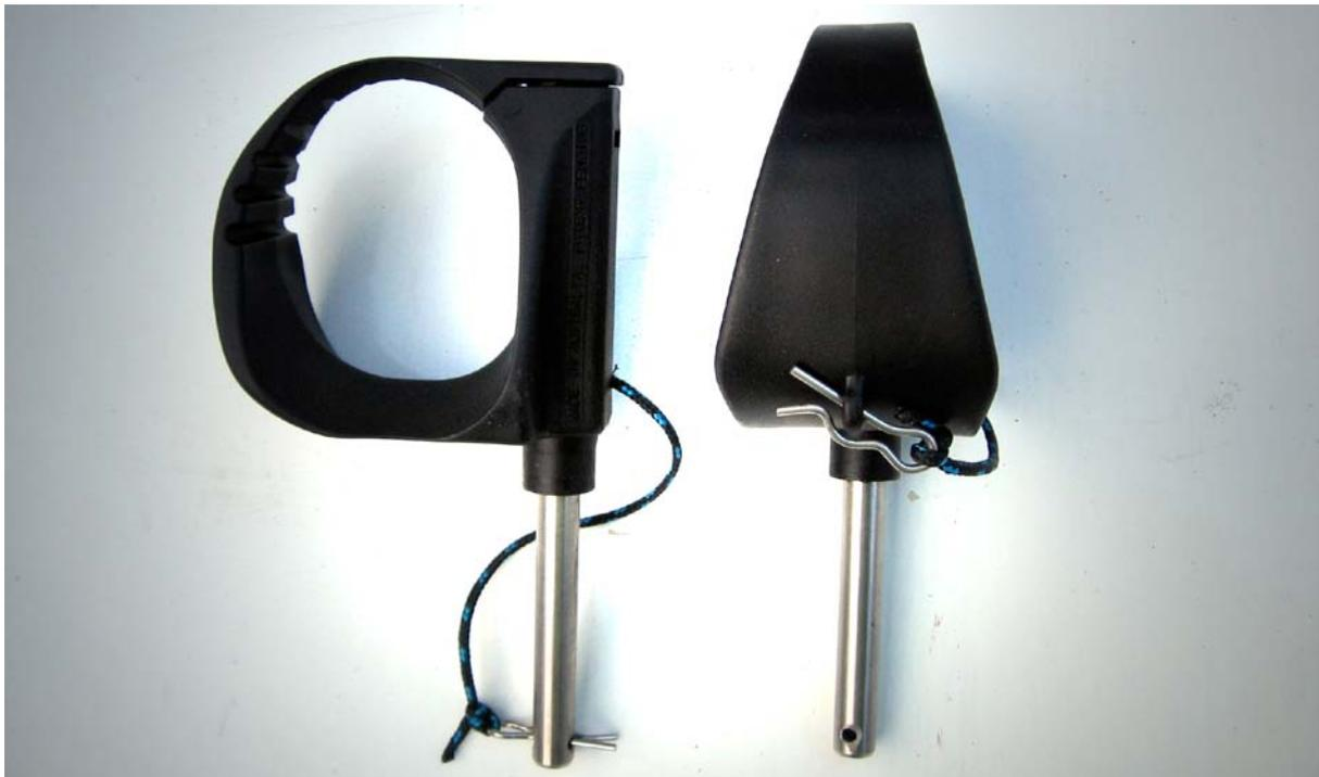
**Retaining pin deployed and stowed. Without such a system the pins will be lost or unavailable when needed.**
