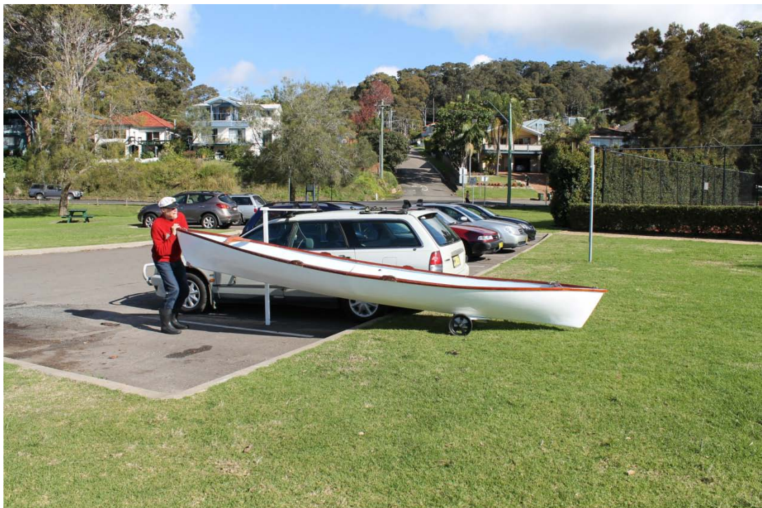
One end of the dory is lifted onto the roof rack extension.
